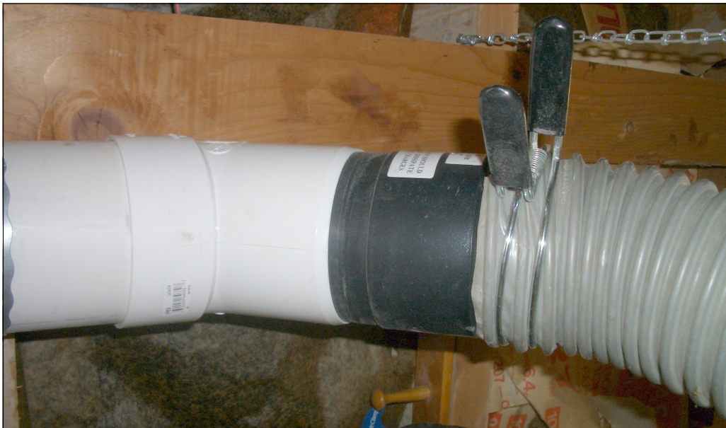
Figure 4 This is a closer view of the main transitions at each end. From left to right, the pipe has the female end of the sewer elbow over it then the splice (turned down in diameter) slipped inside the male end of the sewer elbow. Finally, the hose is installed on the splice and held in place by the squeeze hose clamp.
