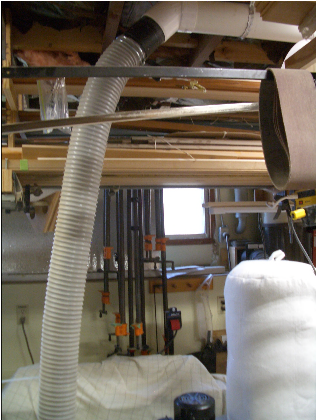
Figure 2 This shows the connection from the dust collector's hose to one end of the pipe and fittings in the ceiling.
