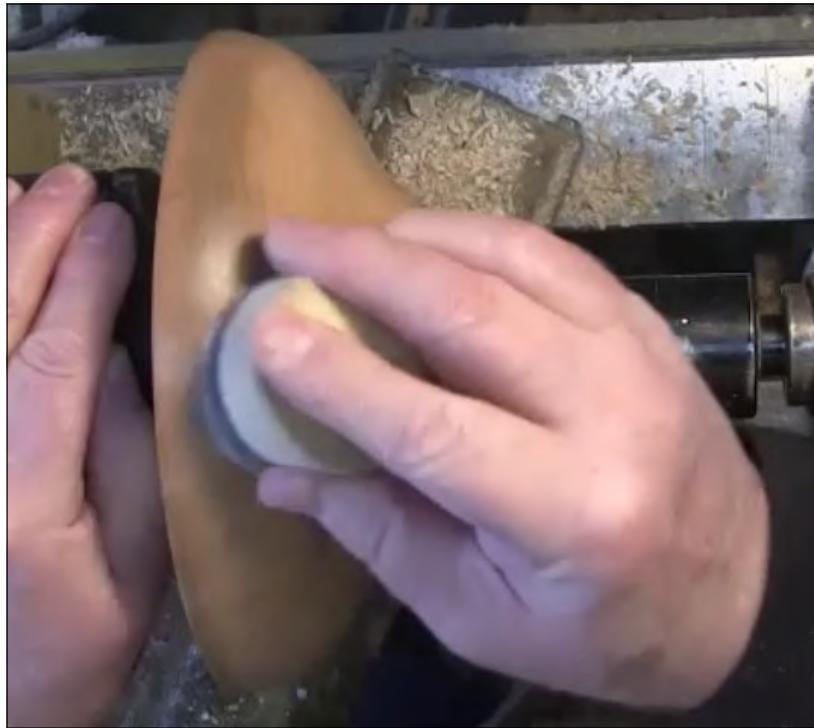
Figure 8 Repair any imperfection before continuing, here orbital sanding with 600 grit Abranet.
