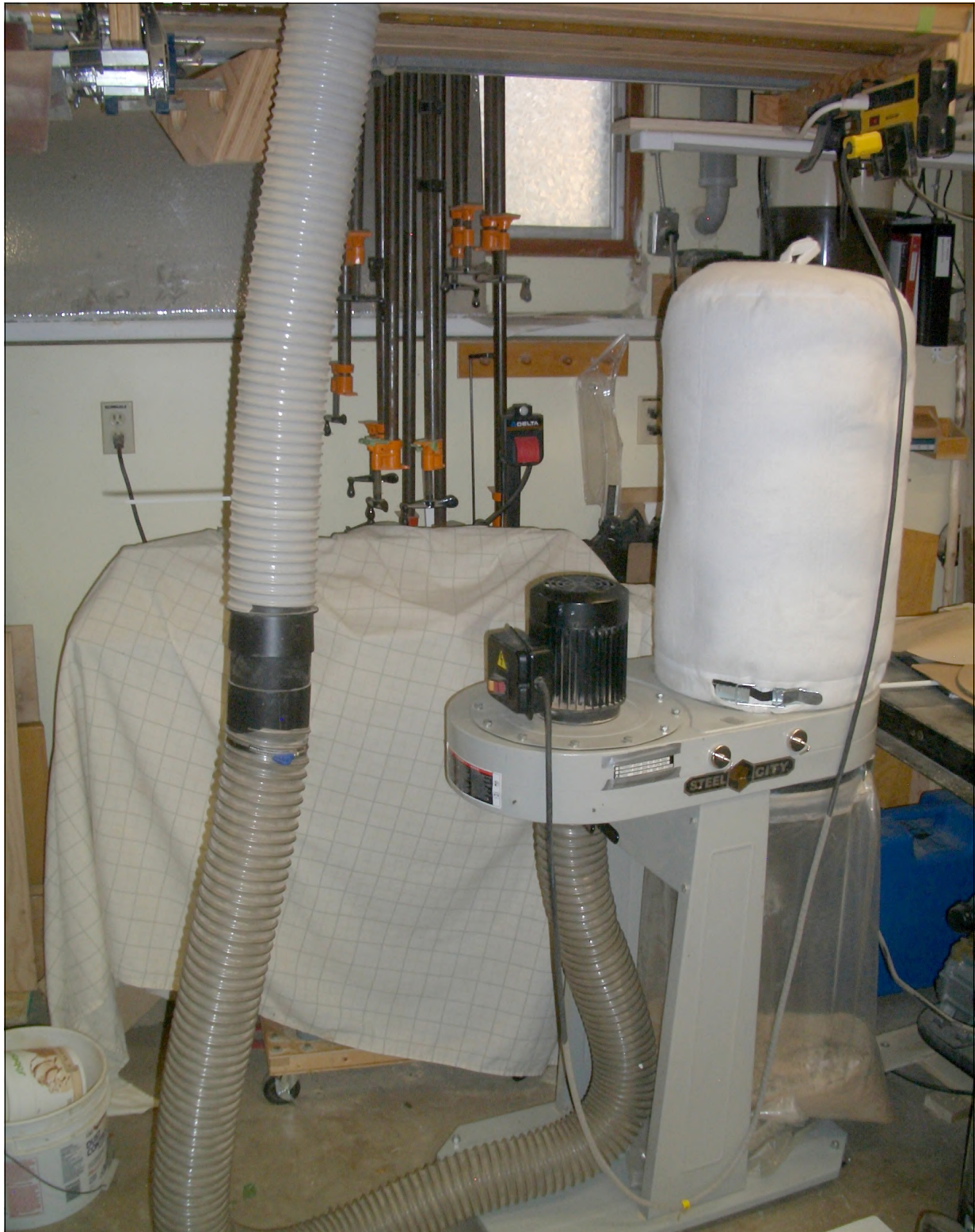
Figure 1 This shows how my dust collector's vacuum is directed up to the PVC pipe in the ceiling.
